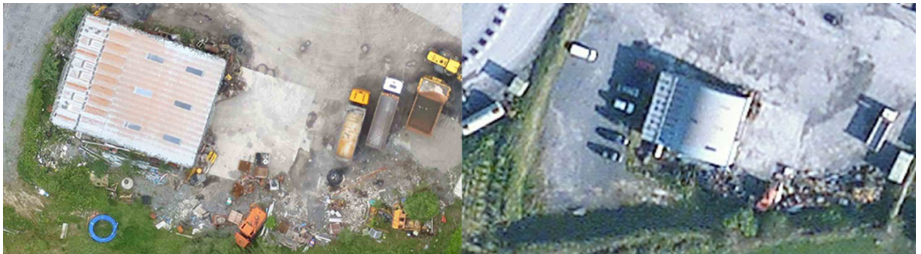
Figure 3: Drone imagery (centimetre resolution per pixel) versus satellite imagery (metre resolution per pixel)
